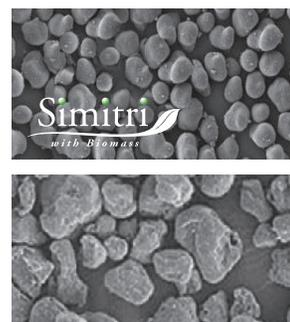
Konica Minolta's exclusive Simitri HD toner formulation uses smaller and more consistent particles, giving B&W reproductions greater detail and sharper, more legible text at 1200 dpi print resolution.
